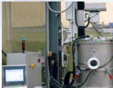
WMH weighing module in an oxide crystal puller system. (Picture: Crystal Growing Systems GmbH, Germany)
