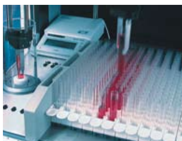
SAG weighing module in a liquid handling system. (Picture: Tecan Schweiz AG, Switzerland)
