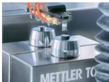
WM weighing modules in a metal powder press for hand metal cutting inserts. (Picture: Fette GmbH, Germany)
