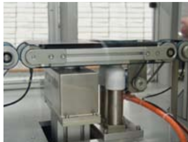
WM weighing modules in a handling machine for solar wafers. (Picture: Jonas & Redmann, Germany)
