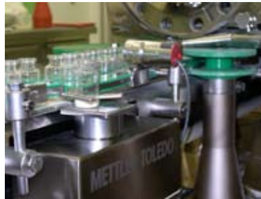
WM weighing modules in a pharmaceutical filling system. (Picture: F. Hoffmann-La Roche AG, Switzerland)
