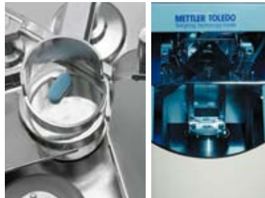
WM weighing modules in tablet checking systems. (Picture: Dr. Schleuniger Pharmatron AG, Switzerland and Sotax AG, Switzerland)
