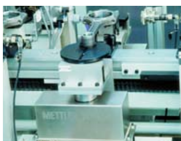
WM weighing module in a taring system for car piston rods. (Picture: Hofmann Mess- und Auswuchttechnik GmbH & Co. KG, Germany)
